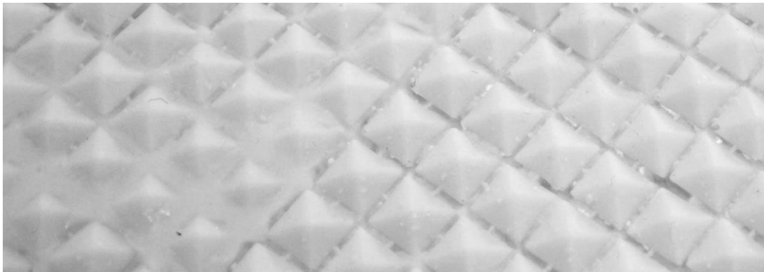
Figure 26 Rubber cast of smaller pyramid shaped elements
