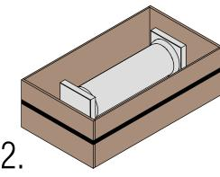
The foam is then placed into a plywood box, held together with a strap.
