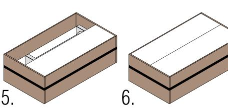
Repeat steps 3 and 4 for the top half. The plaster will be poured into the drilled holes and create a key-like fit when reusing the mold.
