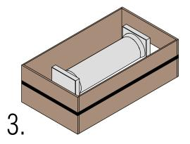
A quarter of the box is blocked off with either clay or a 3D printed piece to fit. Plaster is then poured into this section.
