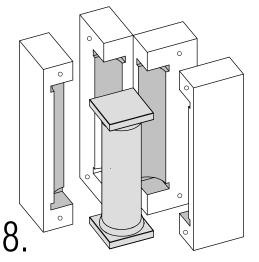
The plaster is then split apart to reveal the final mold.
