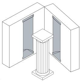
The plaster is then split apart to reveal the final mold.
