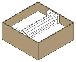
Plaster is poured into the plywood up until about halfway. Once this has dried, vaseline can be used to prevent sticking.
