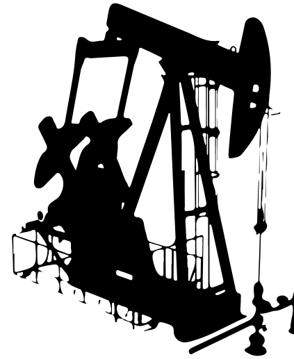
Oil is pumped to the surface by a Pumpjack [Pumpjacks can pump anywhere from 5-40 liters per stroke (1.3-10.5 gallons)] Water/or other gases used in the early processes is pumped into a second hole to increase pressure and move oil up towards the pipe.
