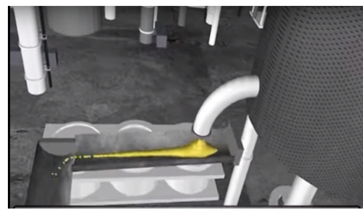
Polymer pellets are melted into a thick liquid plastic the heat needed to melt the pellets can vary from 160 to 700 degrees fahrenheit. The then liquid plastic is then injected into a mould.
