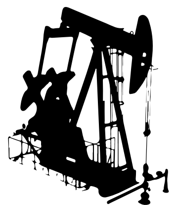
Oil is pumped to the surface by a Pumpjack [Pumpjacks can pump anywhere from 5-40 liters per stroke (1.3-10.5 gallons)] Water/or other gases used in the early processes is pumped into a second hole to increase pressure and move oil up towards the pipe.
