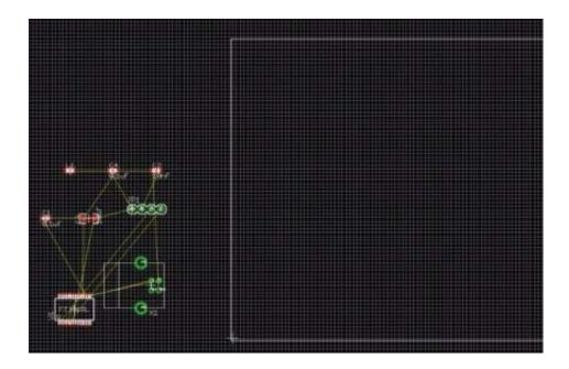
Make sure you're on a 0.1" grid by pressing F10. Then hit F7 and hold control while clicking near the origin. This will grab the frame corner and force it onto the 0.1" grid. Make the bottom left corner sit at (0,0):
