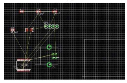
Now go to town bringing the components into the board area. Keep in mind the gold color un-routed 'air' wires. The less twisted you make these by creatively arranging your components, the easier the trace routing will be.
