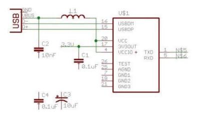
To wire a pin (TXD) to a far point (the 4-pin connector for example), instead of sending a wire half way across the page, we use net names. The green wire is not physically seen on the schematic, but Eagle knows to connect the two points on the layout because the two green wires have the same name.
