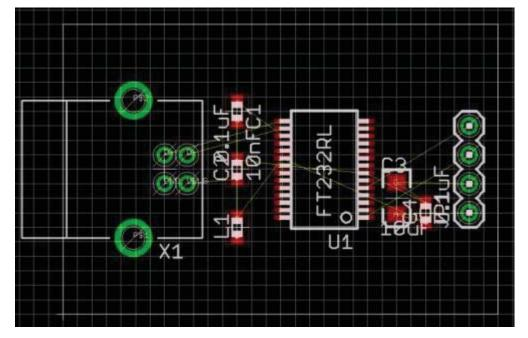
Here are the components arranged in a basic configuration. Another beef I have with Eagle is the default colors for the various layers make it impossible to see what is going to be printed on the silkscreen layer. Let's change the 'tPlace' layer to pure white and change the 'tDocu' layer to lemon yellow.
