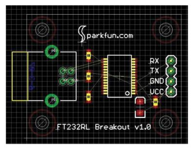
Above is the completed board ready for trace routing.
