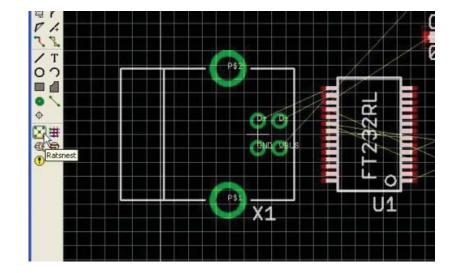
Hit the Ratsnest button from time to time to recalculate the air wires.
