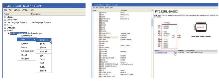
The schematic editor should open. Now go back to the Eagle Control Panel and expand the SparkFun Library: You should see a long list of parts. Highlight the FT232RL-Basic part and in the right screen click on ADD. The schematic editor will pop up allowing you to place the FT232RL.
