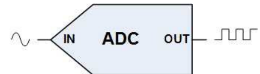
ELECTRICAL SYMBOL FOR ANALOG TO DIGITAL CONVERTER (ADC)
