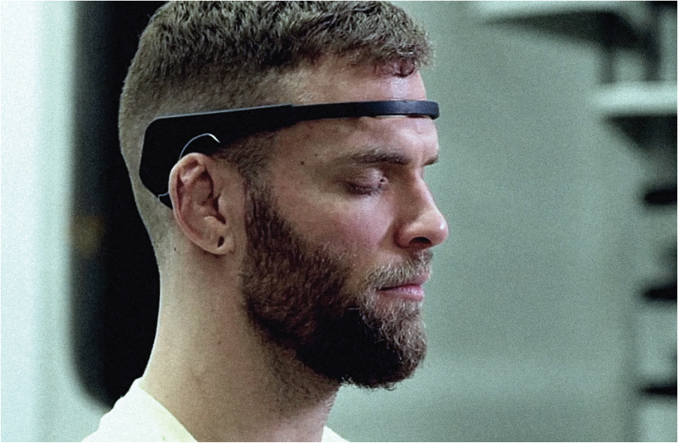
NEUROSKY MINDWAVE MOBILE EEG HEADSET
