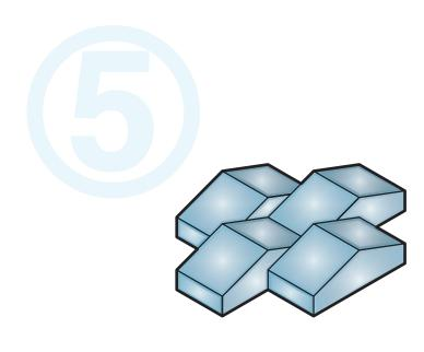
**FINAL TILE** AFTER THE TILE IS HEATED IN THE KILN THE GLAZE AND GLAY ARE BONDED TOGETHER AND REDUCED IN SIZE BY ABOUT 7%
