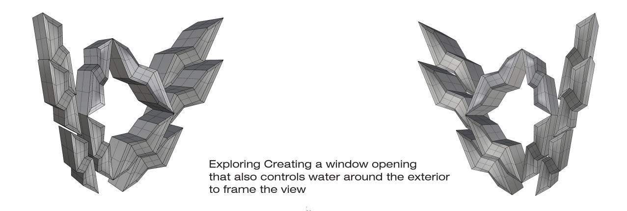
Water flows down the tiles and is deflected by the lip on the edge to control the flow around the opening
